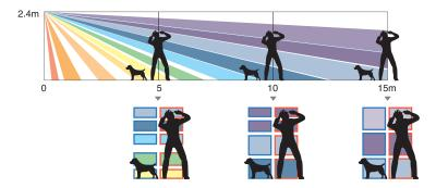
CDX series has 82 dense zones. In the detection coverage, 4 or more zones must be crossed to distinguish between human and small animal detection. In addition, newly developed digital MPU "CORE PLATFORM" provides more accurate detection.
